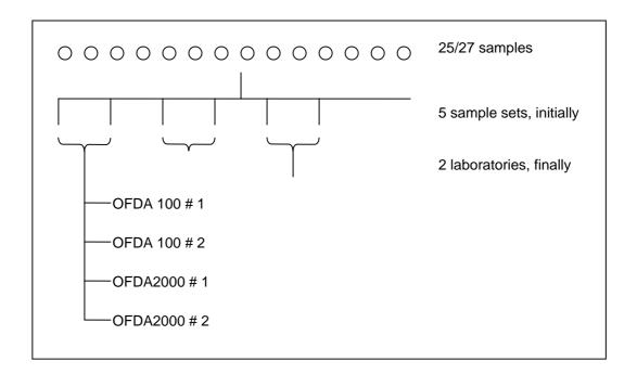
Each subsample was measured using two separate slides, and therefore the total workload included 16 calibrations and validations and over 1600 individual measurements. Each laboratory reported MFD, SD, count and mean curvature on all measurements. No observations were eliminated as outliers and there was only 1 missing value.
