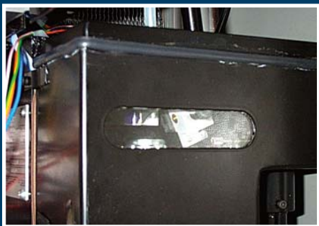
Wire wheel mounted inside the Laserscan optical bench.
