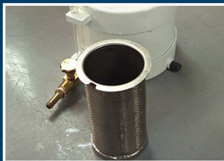
R&D's engineers designed a stainless steel filter to replace the CSIRO's fabric filters in the Laserscan instrument.
