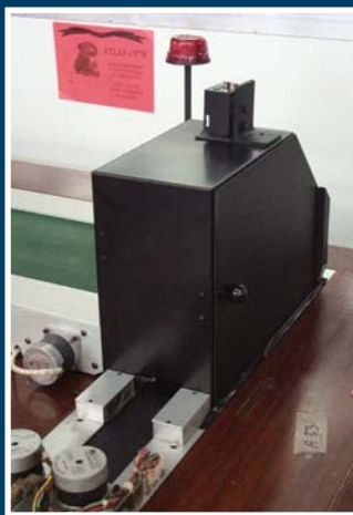
Prototype Crimp Frequency measurement system mounted on an ATLAS instrument.
