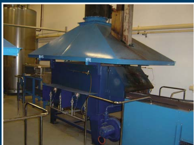
IWTO-19 has been amended to permit the use of Near Infrared Reflectance as replacement for ashing furnaces (above) for determination of residual mineral matter in laboratory scoured wool core samples.
