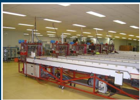
Design modifications to AWT Ltd's MTS machines, which are an integral component in preparing samples for Staple Length & Strength measurement, will make the machines faster and therefore more productive.
